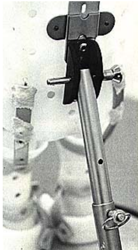
Figure 4. Posterior view of telescoping bar and locking pushpins
